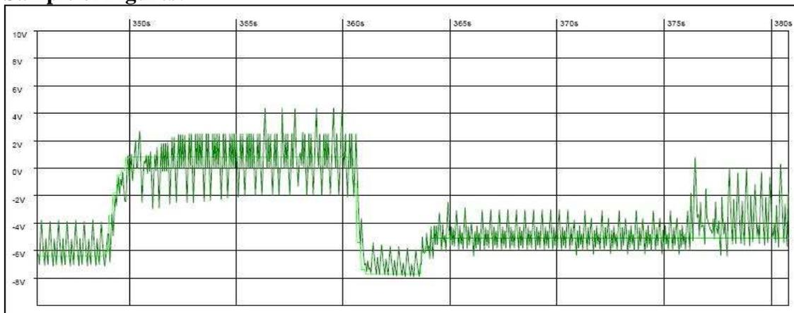
Figure (1): Response of a flow rate due to successive step changes in the set point under PID control action with  $K_c = 15.21$ , integral time constant  $\tau_i = 2.2$  s & and derivative time constant  $\tau_d = 1.2$  s.
